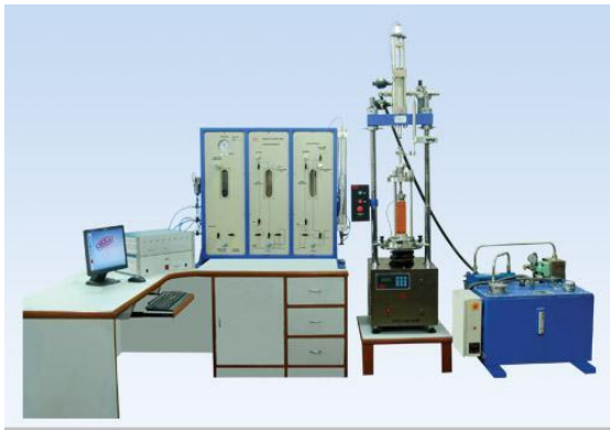
Fig. 2 Cyclic triaxial setup
