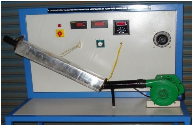
Fig. 2.4 Experimental Setup of Square Cross Section Duct at 45°
