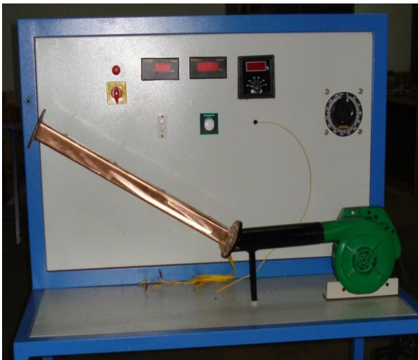
Fig 2.1: Test section copper square duct without insulation and heater
