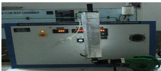
Fig. 2.6 Experimental Setup of Square Cross Section Duct at 90°
