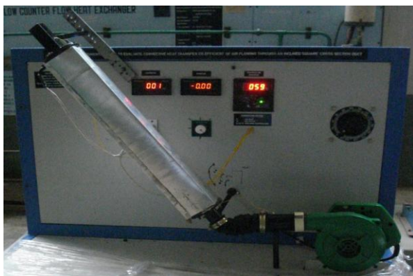
Fig. 2.5 Experimental Setup of Square Cross Section Duct at 60°
