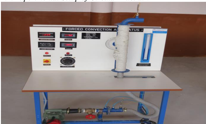
Fig. 2.2 Experimental Setup of Circular Duct at 0°
