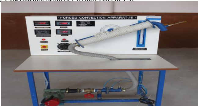
Fig. 2.7 Experimental Setup of Circular Duct at 150°
