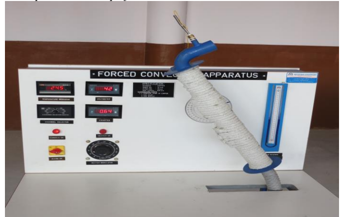
Fig. 2.3 Experimental Setup of Circular Duct at 30°
