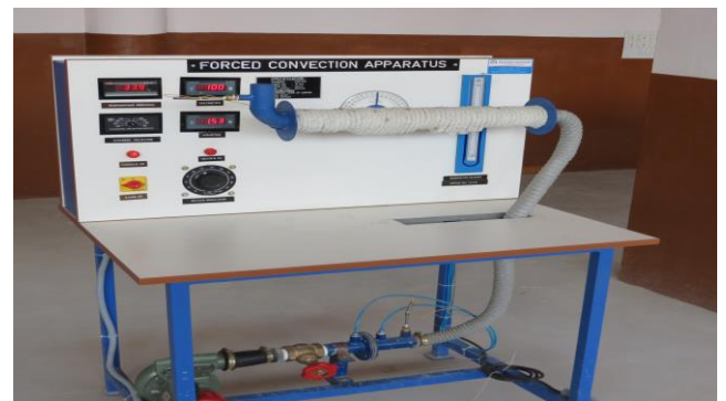
Fig. 2.5 Experimental Setup of Circular Duct at 90°
