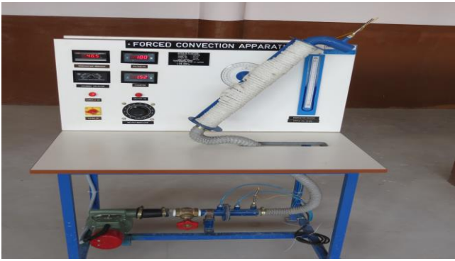
Fig. 2.6 Experimental Setup of Circular Duct at 120°
