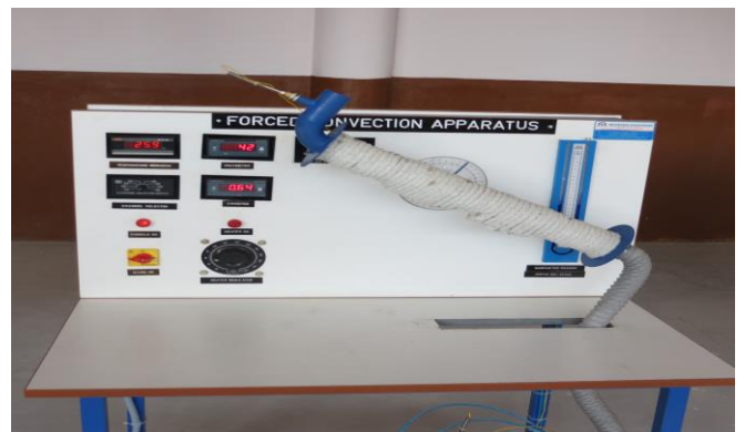
Fig. 2.4 Experimental Setup of Circular Duct at 60°
