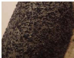
Figure 18. Mud Cake in 10ppb of LCM (COFFEESEAL)
