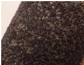
Figure 17. Mud Cake in 15ppb of LCM (COFFEESEAL)
