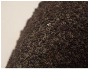
Figure 16. Mud Cake in 20ppb of LCM (COFFEESEAL)
