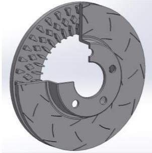
Fig. 2. Section View of Star Pillared Brake Rotor
