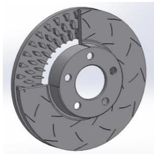
Fig. 3. Section View of T-Pillared Brake Rotor
