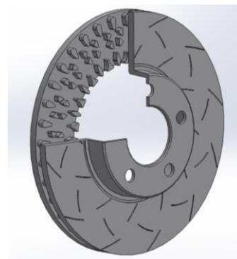
Fig. 1. Section View of Diamond and Tear Drop Pillared Brake Rotor
