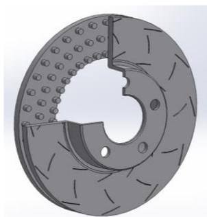
Fig. 4. Section View of Circular Pillared Brake Rotor
