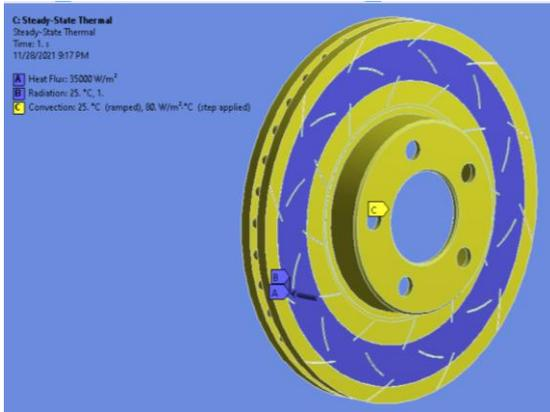
Fig. 13. Boundary conditions for Static Thermal Analysis
