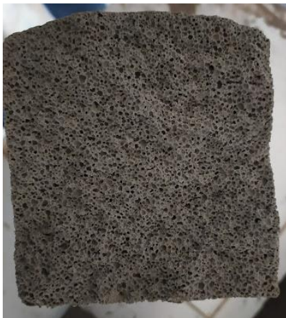
Fig.2 NAAC Block with 20% replacement of BA with FA
