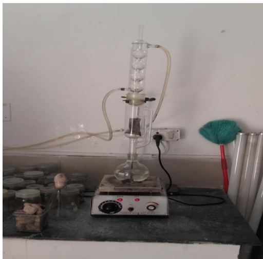
Fig. 5 Soxhlet extractor for methanol extraction
