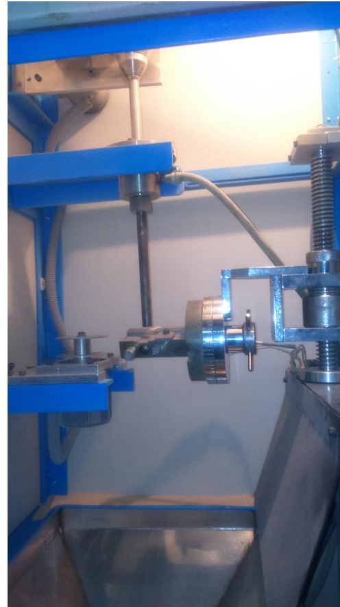
Fig 2. Actual image of air jet erosion testing rig
