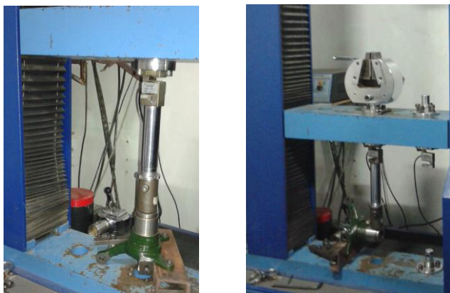
a) Lateral force(8.44KN) b) Longitudinal force(6.85KN) Fig.11 Loading conditions for steering knuckle
