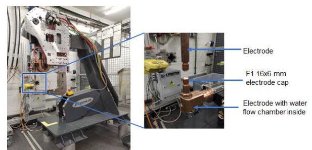
Figure 1: Fronius 'C-type' resistance spot welding machine along with F1 16x6 mm electrode caps
