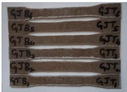
Fig.2: Tensile test specimens of hybrid jute/glass laminated dry
