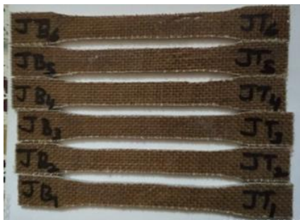
Fig.1: Tensile test specimens of natural jute laminated dry composite.
