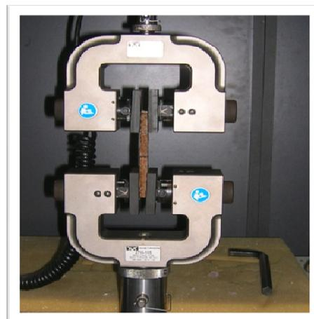
Figure 1: Tensile testing of Composite
