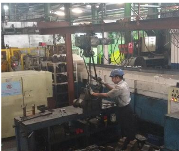
Fig. 8 Moving the retainer assembly to the worktable
