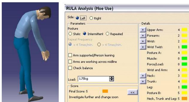
Fig. 6 Virtual Model of Hoe using position and RULA result of the posture
