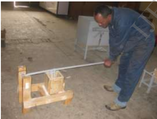
Figure 5. Simple lever based kocho press.
