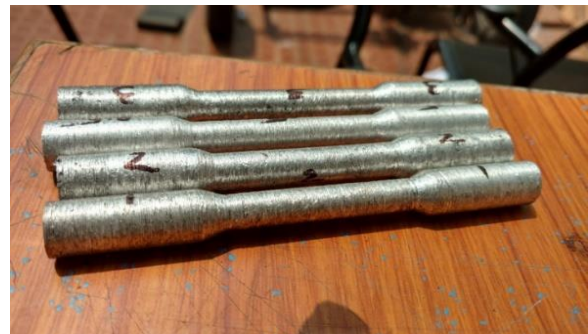
Fig 4. Tensile test specimens (length =57mm, diameter at ends= 12mm and diameter at center =8mm).
