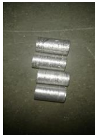
Fig 5. Compressive strength test specimens (Length = 20mm, Diameter = 10mm)
