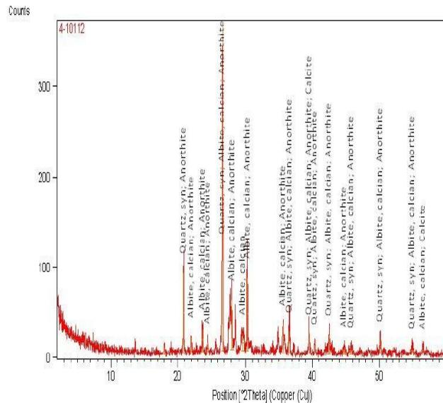
Fig 23. XRD shows results of curing concrete during 28 days concrete with Nano-SiO<sub>2</sub>
