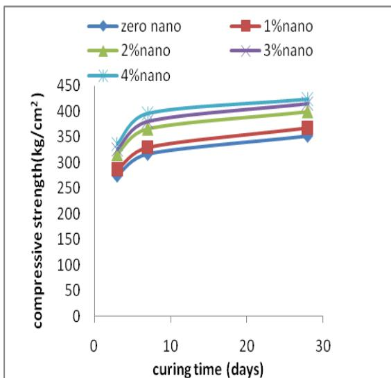
Fig 2. Compressive strength of specimens containing Nano-SiO<sub>2</sub> particles with curing time.
