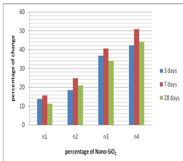
Fig 5. Percentage of increase in flexural strength of cement mortars containing different Nano-SiO<sub>2</sub> percentages at different ages
