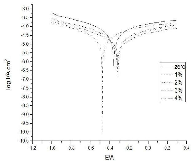
Fig 10. Different concentrations of the Nano-SiO<sub>2</sub> ranging from 1% to 4% at 6 months (first group)
