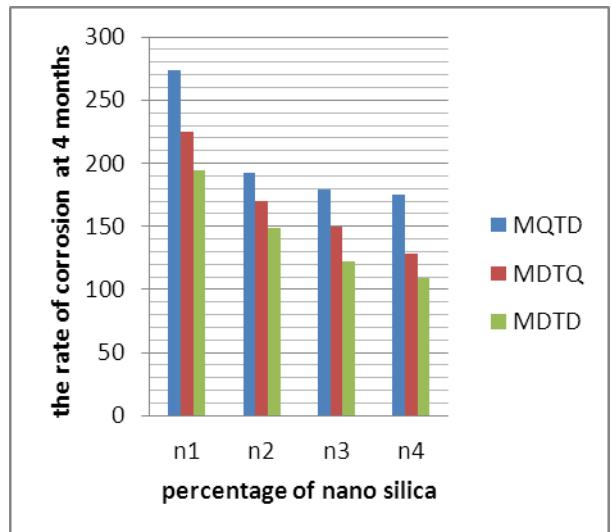
Fig 18. comparison of rate of corrosion at different cases with 1,2,3,4 % Nano-SiO<sub>2</sub> at 4 months
