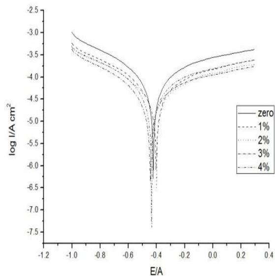
Fig 14. Different concentrations of the Nano-SiO<sub>2</sub> ranging from 1% to 4% at 2 months (third group)
