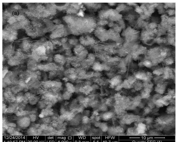
Fig 21. (a) SEM of control sample of concrete
