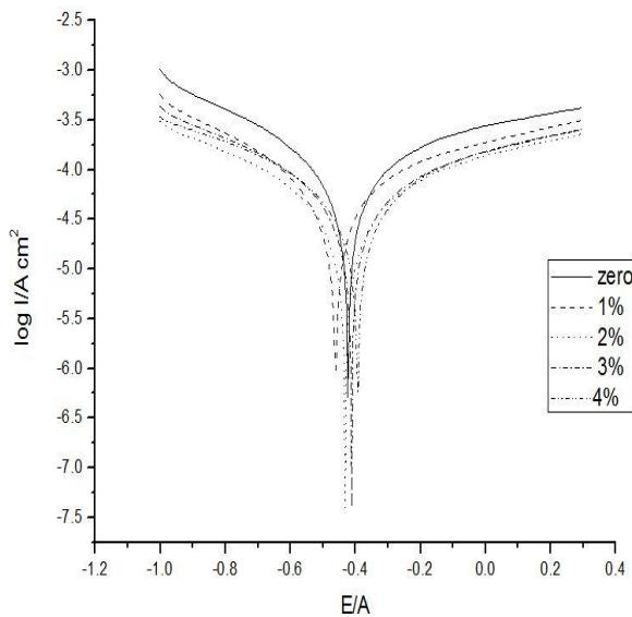
Fig 9: Different concentrations of the Nano-SiO<sub>2</sub> ranging from 1% to 4% at 4 months (first group)
