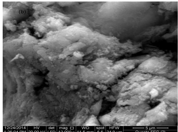
Fig 20. (b) SEM of cement mortar containing Nano-SiO<sub>2</sub>
