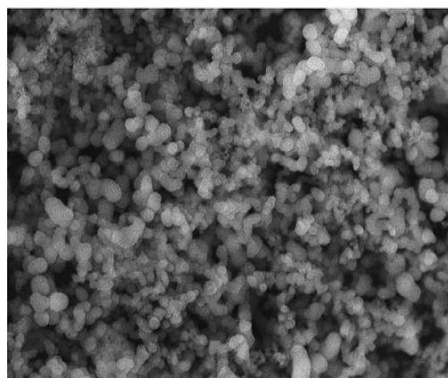
Fig 1. SEM of Nano-SiO<sub>2</sub>.
