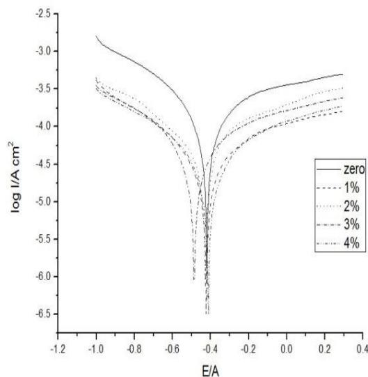
Fig 15. Different concentrations of the Nano-SiO<sub>2</sub> ranging from 1% to 4% at 4 months (third group)
