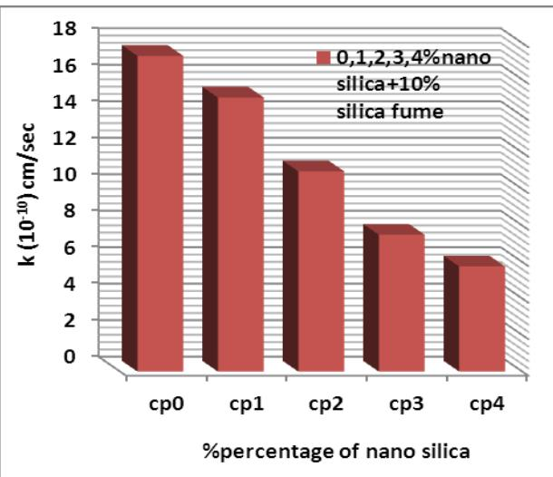
Fig 6. permeability test results of specimens containing 0, 1, 2, 3and4 % Nano-SiO<sub>2</sub>
