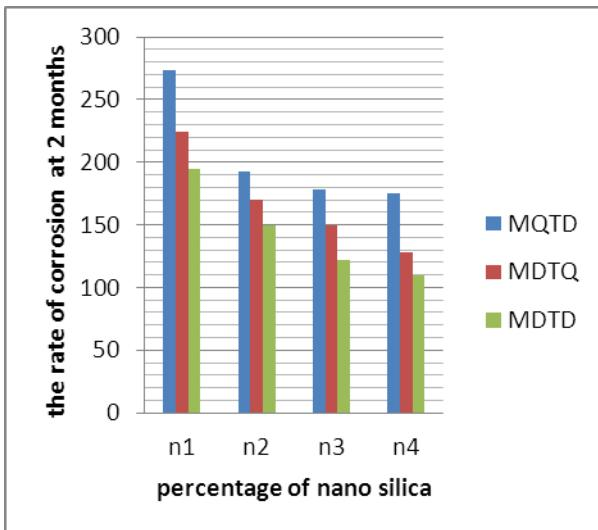
Fig 17. comparison of rate of corrosion at different cases with 1,2,3,4 % Nano-SiO<sub>2</sub> at 2 months
