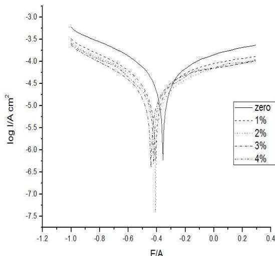
Fig 16. Different concentrations of the Nano-SiO<sub>2</sub> ranging from 1% to 4% at 6 months (third group)
