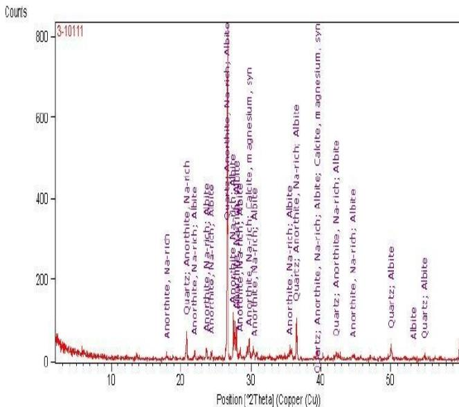
Fig 22. XRD shows results of curing concrete during 28 days
