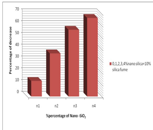
Fig 7. Percentage of decrease in permeability test at different Nano-SiO<sub>2</sub> percentages
