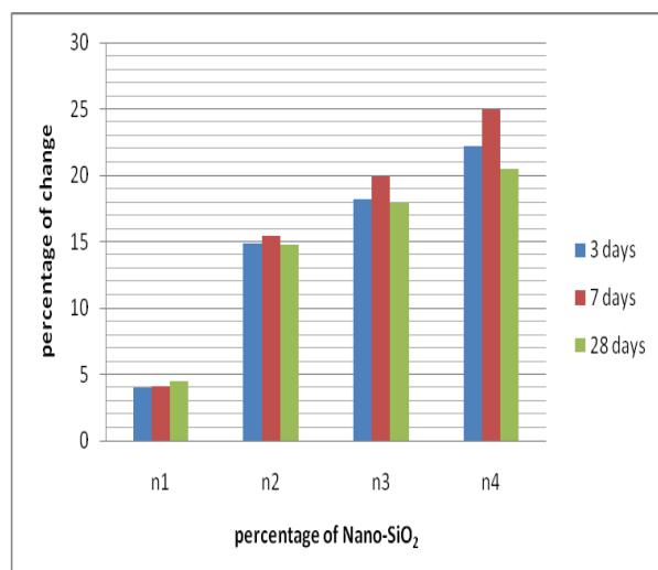
Fig 4. Percentage of increase in compressive strength of cement mortars containing different Nano-SiO<sub>2</sub> percentages at different ages
