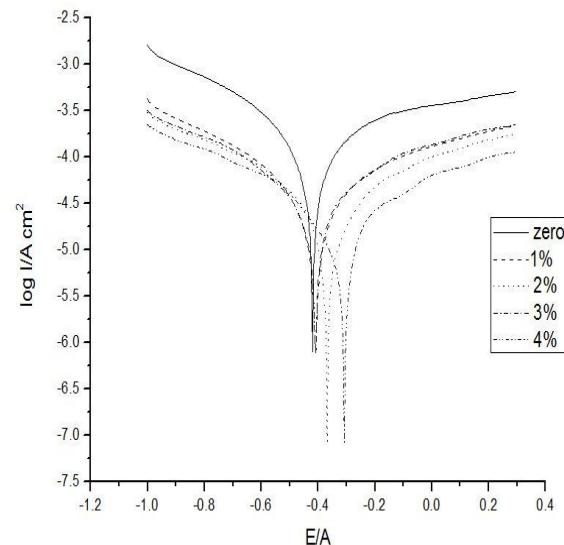
Fig 11. Different concentrations of the Nano-SiO<sub>2</sub> ranging from 1% to 4% at 2 months (second group)
