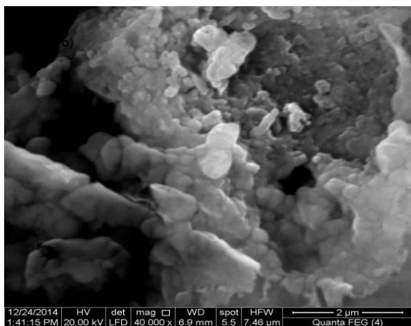
Figure 21: (b) SEM of concrete sample containing Nano-SiO<sub>2</sub>
