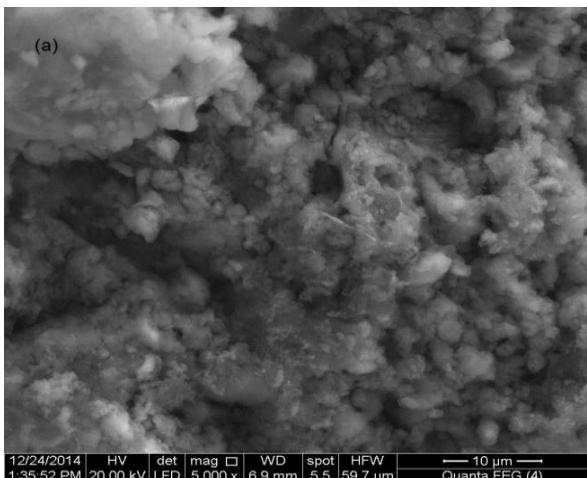
Fig 20. (a) SEM of ordinary Portland cement mortar
