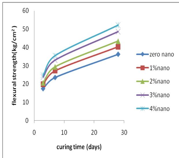
Fig 3. flexural strength of specimens containing Nano-SiO<sub>2</sub> particles with curing time.
