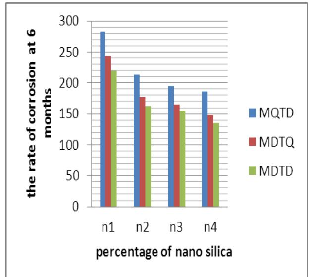
Fig19. comparison of rate of corrosion at different cases with 1,2,3,4 % Nano-SiO<sub>2</sub> at 6 months
