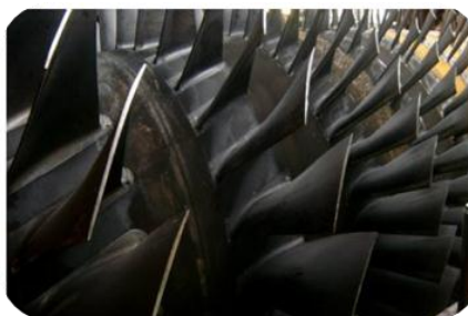
Fig. 1. Black deposits on compressor blades caused by hydrocarbon contaminants [11]
