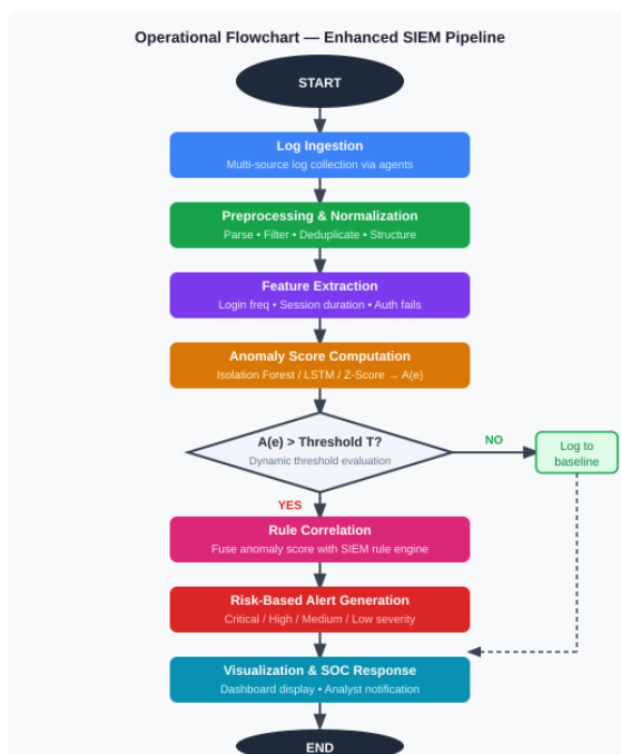
Fig. 2. Flowchart of the operational process of the improved SIEM with anomaly detection pipeline.
