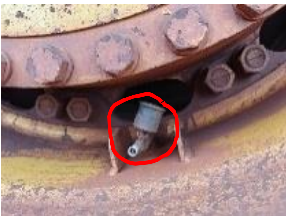
Fig-7: Sensor fitted in the Tyre Valve
