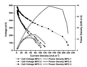
Figure 1. MFC polarization curves and power density for MFC-1, MFC-2 and MFC-3
