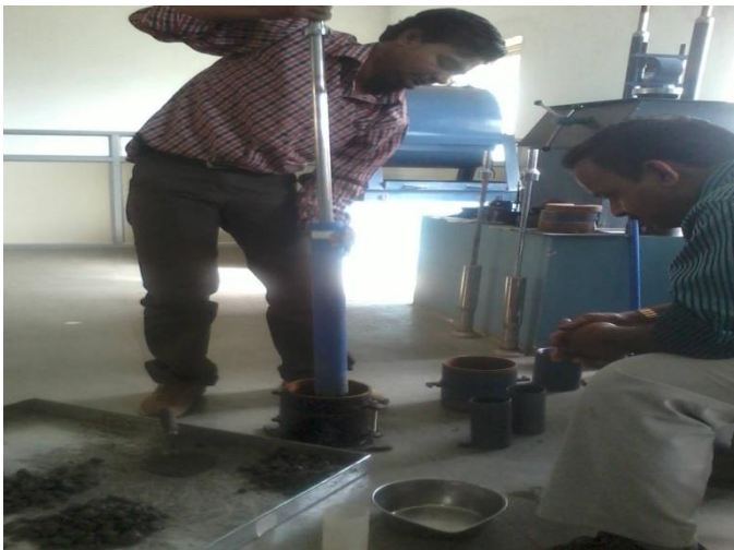
Proctor test for unit weight of fresh pervious concrete
