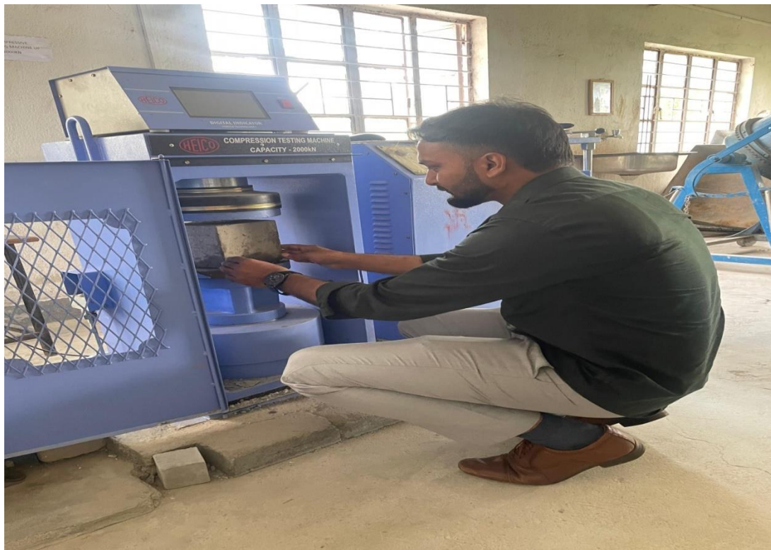
Fig. 4.3: Compressive strength testing
