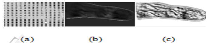
Fig. 3. Image enhancement. (a) Image subblock. (b) Background estimated finger vein image. (c) Image after local histogram equalization.
