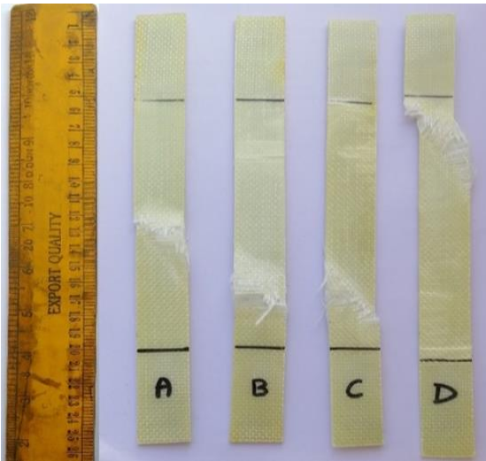
Fig. 3. Failed configurations of (a) Unmodified GFRP (b) 0.1 % nano- \text{Al}_2\text{O}_3 (c) 0.3% nano- \text{Al}_2\text{O}_3 and (d) 0.5 % nano- \text{Al}_2\text{O}_3
