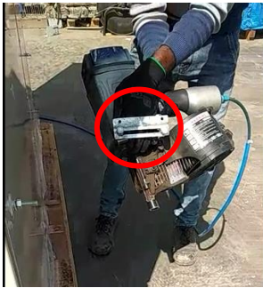
Fig. 3 After Kaizen implemented on Coil nail Machine
