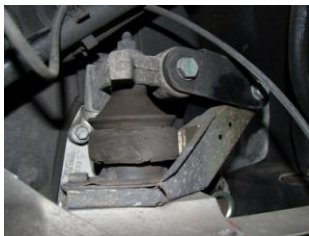
Fig 4 Engine Mounted on Engine Mount
