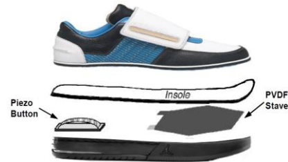
Fig. 2 First prototype of the energy generator. Two piezoelectric polymer films above the sole.
