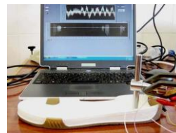
Fig. 10 Performance test. A handspike system was used in order to apply constant pressure impulses to the sole.
