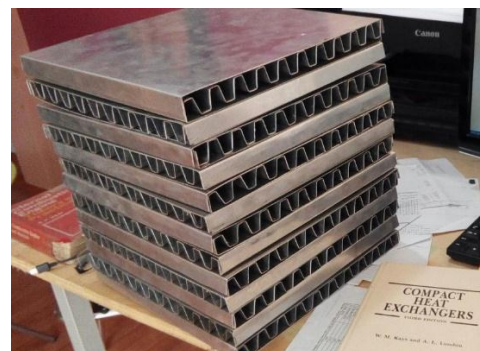
Figure 3. Cross flow plate fin heat exchanger
