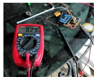
Fig. 14. Current Consumption of The Device During Sleep Mode
