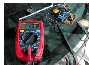
Fig. 13. Current Consumption of The Device When Powered-ON
