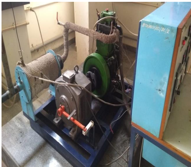
Fig -4: Photographic view of 4-Stroke Single Cylinder Engine
