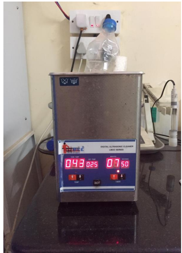
Fig -2: Mixing of Graphene Nano Additives with B20 Blend
