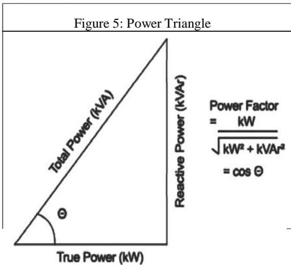
The active power (shaft power required or true power required) in kW and the reactive power required (KVAR) are 90° apart vector in a pure inductive circuit, i.e., reactive power KVAR lagging the active kW. The vector sum is called the apparent power or KVA, as illustrated above and the KVA reflects the actual electrical load on distribution system (Brown, 2008).
