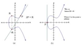
To double a point P to get R, i.e. to find R=2P, consider a point P on an Elliptic Curve as shown in figure (a). If y coordinate of the point J is not zero then the curve line at P will intersect the elliptic curve at accurately one more point -R. The reflection of the point -R with respect to x-axis gives the point R, which is the result of doubling the point R.
