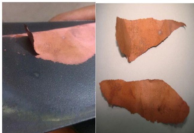
Figure 7: Copper deposition on DSA
