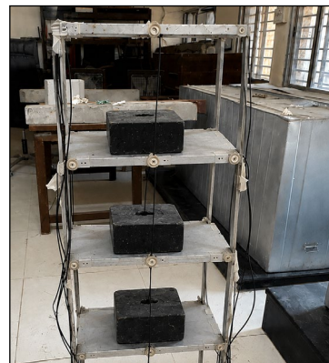
Fig 3: Mass Addition Damage Condition
