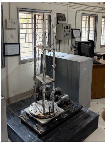
Fig 1: Experimental Steel Frame Structure Used for EMI Analysis
