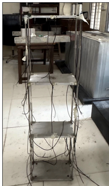
Fig 4: Partial Bolt Removal Damage Condition
