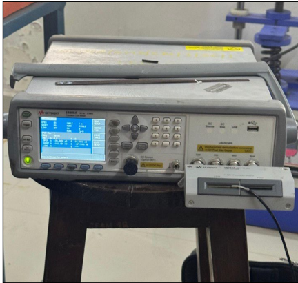
Fig 5: Experimental Setup for EMI Data Acquisition Using LCR Meter
