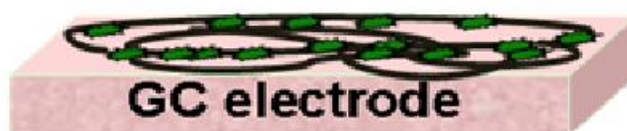
Scheme-1: Schemetic representation of CNT-phthalocyanine electrode.
