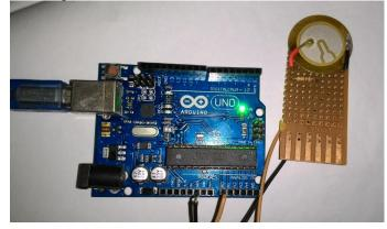
Now the program is uploaded to the Arduino. The sensor starts sending in data to the Arduino , which can be seen from the Serial Monitor. The Serial Monitor can be accessed from the Tools menu of the Arduino IDE.
