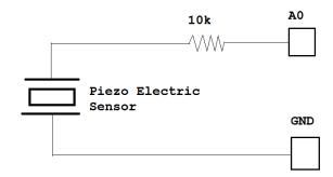
In the above circuit diagram A0 acts as the analog input on the Arduino board. GND serves as the ground pin of the Arduino.
