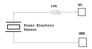
In the above circuit diagram A0 acts as the analog input on the Arduino board. GND serves as the ground pin of the Arduino.
