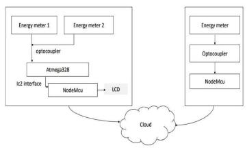
We have mainly two section, one is consumer section and other is power station section. In consumer section we have two energy meter, optocoupler, Atmega 328,ic2 interface, Node mcu, and LCD.Our proposed system can be placed either in existing energy meter or can be placed separately.
