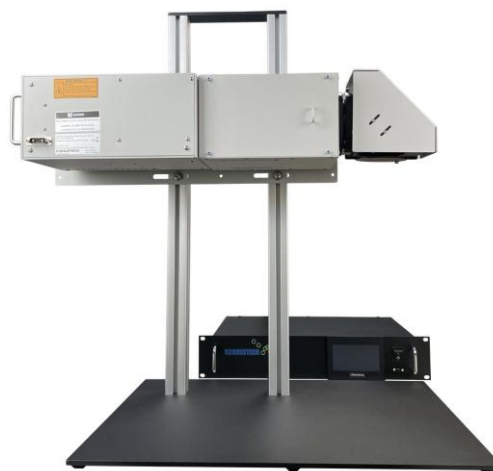
Figure 3. AM1.5G simulated solar illumination system employed for photovoltaic characterization.
