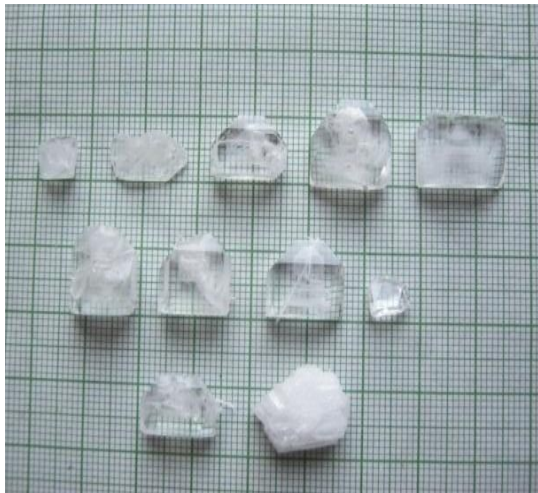
Figure 1. Photograph showing sample crystals grown. [Top row: from left are ZTS1,ZTS2,ZTS3,ZTS4, ZTS5, Middle row: from left are ZTS6, ZTS7, ZTS8, ZTS9, Bottom row: from left are ZTS and MTS ]
