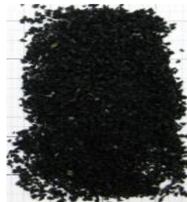
Fig 2. Fine Crumb Rubber Aggregates
