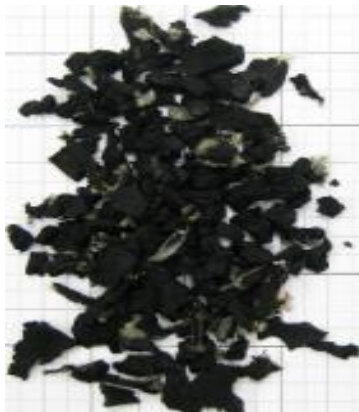
Fig 1. Coarse Crum Rubber Aggregates
