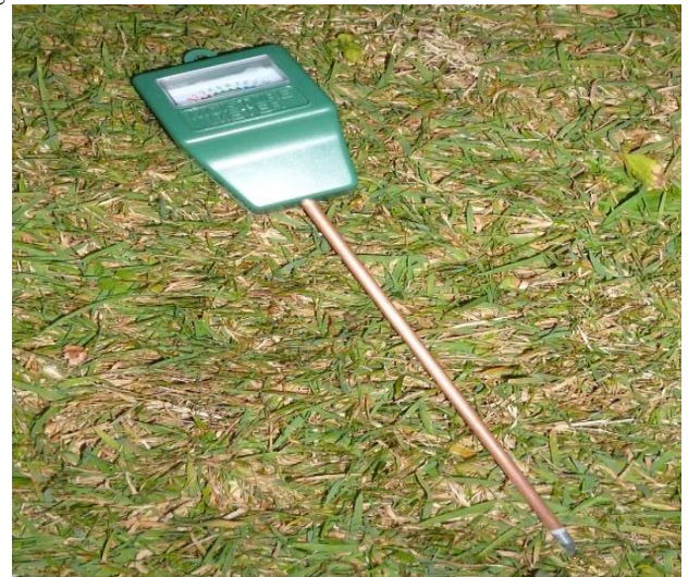
Fig. 5. Soil moisture sensor
