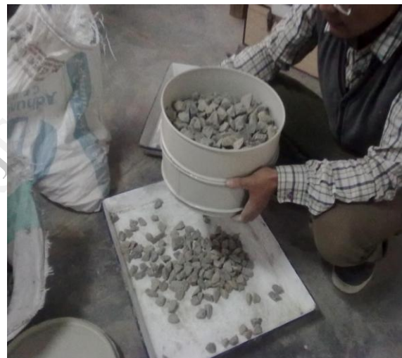
Photo 2: Sieve analysis of 20 mm aggregate
