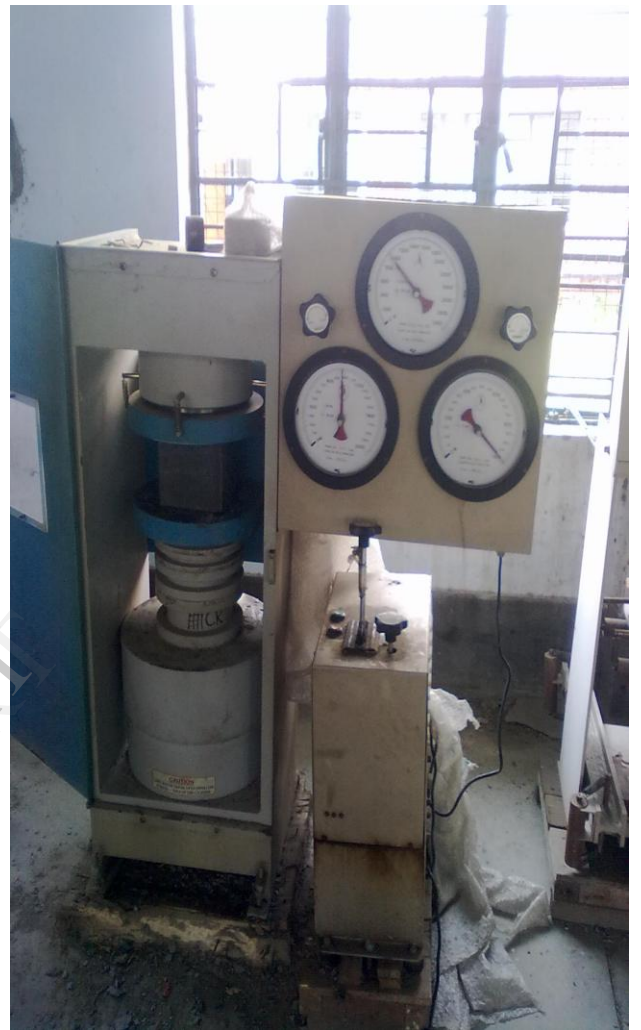
Photo 7: Testing of plain concrete and SFRC cubes in the CTM (compressive testing machine)
