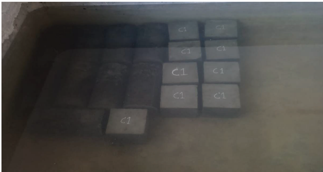
Fig.5.1 Immersion curing method
