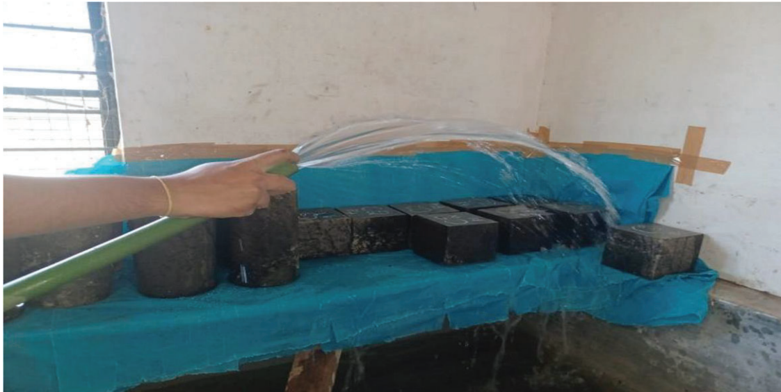
Fig.5.2 Sprinkling of water method
