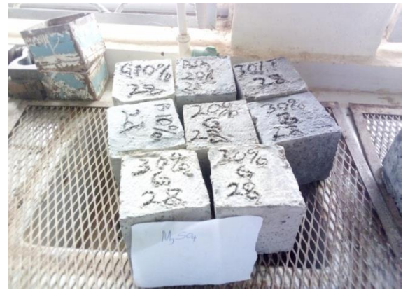
Fig 1. Specimen in MgSO 4 solution at 28-days
