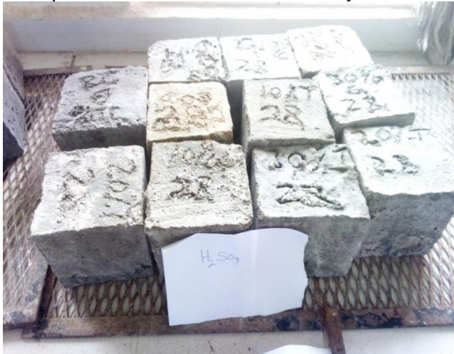
Fig 3. Specimen in H_2SO_4 solution at 28-days
