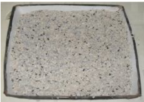
FIG 3 Reinforcement particles- size 2 mm
