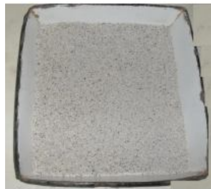
FIG 5 Reinforcement particles- size 425 microns
