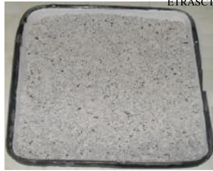
FIG 4 Reinforcement particles- size 1.18 mm
