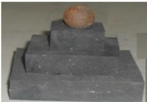
FIG 2 Square footings, sides 6.5 cm, 4.5 cm & 2.5 cm
