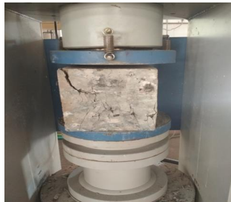
Fig 2: Failure of Cube.
