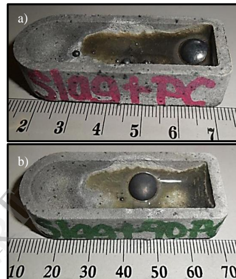
Fig. 8: Nature of metal produced from reduction of slag by (a) Pet coke and (b) Blend 1
