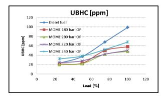
The ignition delay period of the fuel at lower IOP is high. This results in sudden combustion of the fuel, which results in higher UBHC emission. Among the IOPs, the IOP of 200 bar results in lower UBHC emission. But at 75 and 100% of full load, the difference in UBHC of 200 and 220 bar is negligible. The engine emits lower UBHC emission with the MOME as compared to the diesel. At low loads, there is small difference in the UBHC of MOME and diesel, but at higher loads, the difference is high.
