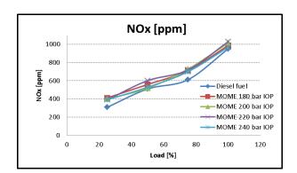
From the figure, it is observed that the IOP of 200 and 220 bar results in higher Nox emission. This is due to the better atomization and combustion of the MOME, which results in higher combustion temperature and hence higher Nox emission. It is observed that the higher injection pressure results in higher Nox
