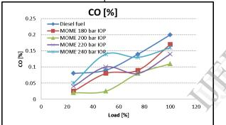
This is due to the presence of oxygen in the molecular structure of the MOME, which results in better combustion and reduces the CO emission.
