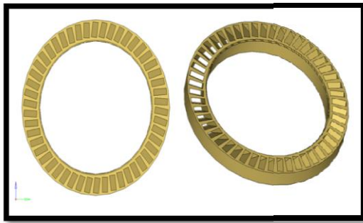
Figure 3.1 CAD Detail of Swirler Baseline Configuration with Straight Passage.
