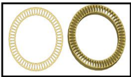
Figure 3.3 CAD Detail of Swirler Configuration-B with Elliptical Passage. The above figure shows configurations B of swirler used for the computational investigation and performance comparison of combustor. It has a 60 elliptical passage in which one length is L1- 10mm and L2- 4mm. Configuration B is totally a different swirling passages when compared with the conventional straight passages, Configuration B
